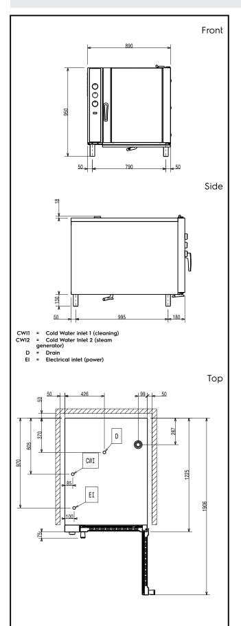
**Electric** Supply voltage: 380-400 V/3N ph/50 Hz Auxiliary: 0.5 kW Electrical power, max: 24.5 kW Capacity: Trays type: 10 (GN 2/1) **Key Information:** External dimensions, Width: 890 mm External dimensions, Depth: 1215 mm External dimensions, Height: 970 mm Net weight: 147 kg Height adjustment: 80/0 mm Functional level: Basic Cooking cycles - air-convection: 300 °C **ISO Certificates**
